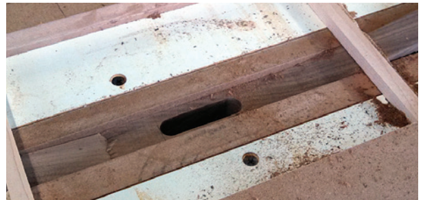
Figure 4: Close-up of headboard clamped for routing spoke mortise
