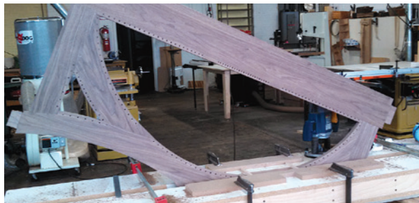
Figure 3: Headboard clamped for routing spoke mortise photo by Chris Pinchbeck
